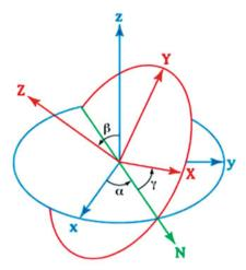
**Fig. 19.5** Euler angles. A passive rotation of  $\alpha$  about the z axis takes the axes (x, y, z) into (x', y', z). This is followed by a passive rotation of  $\beta$  about the y' axis that takes the axes (x', y', z) into (x'', y', Z) and a passive rotation of  $\gamma$  about the Z axis that takes the axes (x'', y', Z) into (X, Y, Z). The vector  $\mathbf{N}$  that lies along the intersection of the xy and xy planes is referred to as the *line of nodes*
