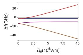
**Fig. 21.4** Frequency shift  $\Delta f$  in GHz of the n=2,  $\ell=1$  states of hydrogen as a function of electric field amplitude in units of  $10^5 \, \text{V/m}$
