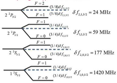
Fig. 21.2 Hydrogen hyperfine structure for the n=1 and n=2 states (not to scale) with splittings  $\delta f_{n,\ell,j}$
