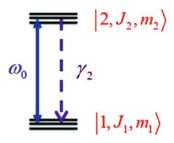
Fig. 24.2 Spontaneous emission between an excited and ground state manifold of levels
