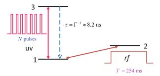
**Fig. 24.4** Level scheme for Problem 24.14. Level 3 is the  $2^2P_{3/2}$  that decays back to level 1. The parameters shown refer to the article of Itano et al. In their experiment the uv pulse width was 2.4 ms and up to N = 64 pulses were used
