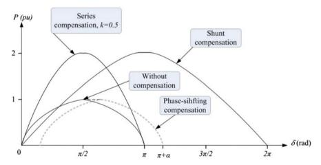
Fig. 8.11 Power transfer characteristics for several compensation cases
