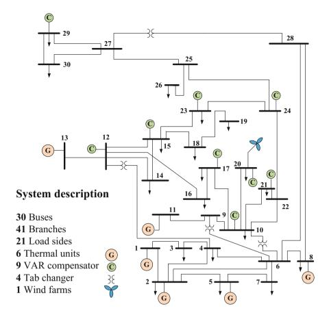
Fig. 12.6 One-line diagram of IEEE 30-bus test system
