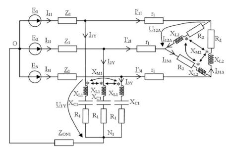
Fig. 1.6 Symmetrical and balanced three-phase system
