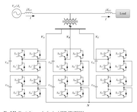
Fig. 8.23 Circuit diagram of a five-level CHB STATCOM
