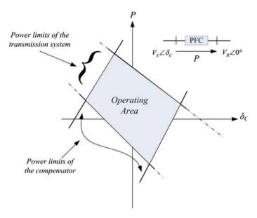
Fig. 8.13 Operating area of a power flow controller (PFC) in the power controller plane
