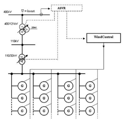
Fig. 6.12 ASVR integration in electrical network
