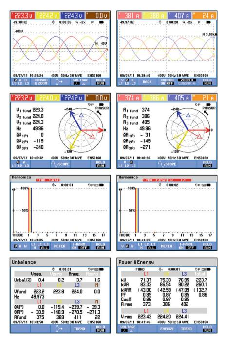
Fig. 2.26 The energy quality parameters of the industrial consumer under investigation
