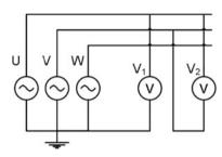
voltmeter  $V_2$  measures the phase voltage between the phases U and the common point.
