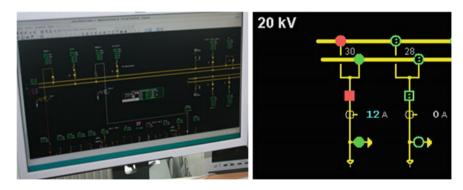
Fig. 15.20 Medium-voltage EPS based on RESs represented in the existing SCADA system
