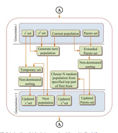
Fig. 9.13 Sub-algorithm of A for design procedure delineated in Fig. 9.12
