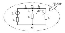
From the above system by summing up the first equation and the second equation multiplied by (j), and the third equation multiplied by (-j) and the fourth equation results the equation of NM expressed at node 1
