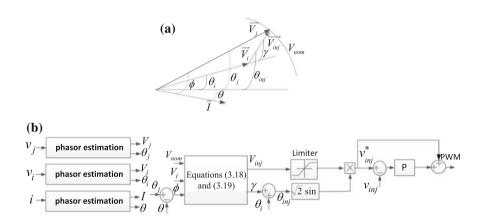
Fig. 3.15 Voltage control based on phasor estimation by series compensator, a vector diagram of the voltages and current during compensation, b block diagram of the control scheme
