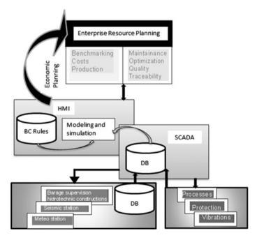
Fig. 15.1 Extended SCADA architecture with application in hydro-energetics
