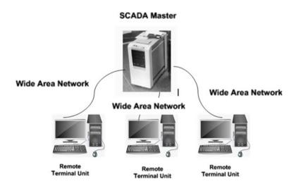
Fig. 15.6 First generation of SCADA systems
