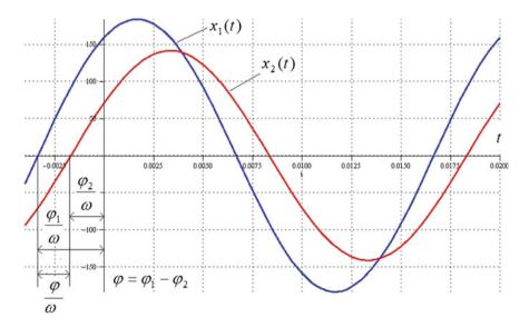
Fig. 2.2 The phase-shift between two sinusoidal signals
