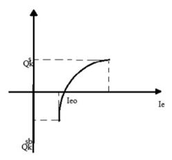
power to their load. In some power plants the hydro units are designed to permit the generator to function without its mechanical power source simply to provide the reactive power capability to the power system [10]. These hydro units work as a compensators when the active power generation is not necessary, Fig. 6.4.
