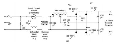
Fig. 4.35 Example of passive PFC [70, 71]
