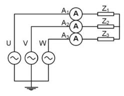
**Fig. 1.17** Current measurement for a three-phase balanced circuit
