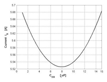
Fig. 4.3 Current  $i_S$  versus value of compensation capacitor  $C_{CO}$  (Example 4.1)
