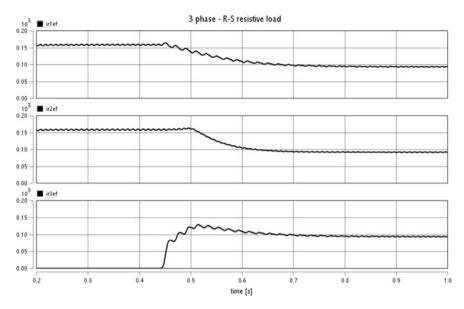
**Fig. 4.24** Time evolution of RMS currents in circuit according Example 4.4, before and after compensation. Compensation parts are connected in time  $\geq 0.44$ . From *top* to *bottom*: RMS currents  $i_R$ ,  $i_S$ ,  $i_T$
