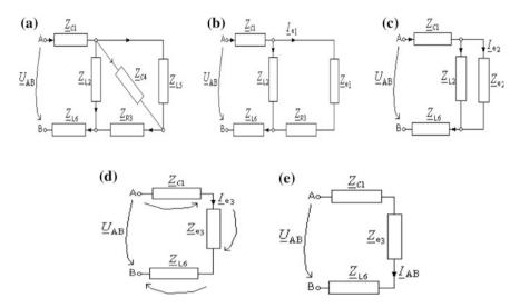
Fig. 2.10 The equivalent AC circuit
