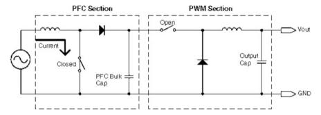
Fig. 4.40 Energizing the PFC Inductor [85]
