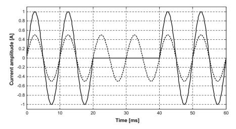
**Fig. 4.33** Burst-Fired waveform test. *Solid line*—test waveform, *dash line*—reference waveform. Test waveform is on for 2 cycles and off for 2 cycles
