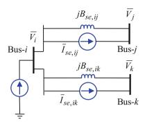
**Fig. 9.8** Voltage source model of GUPFC
