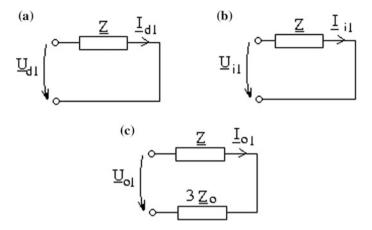
Fig. 1.12 Single phases of a positive, b negative, and c zero-sequence
