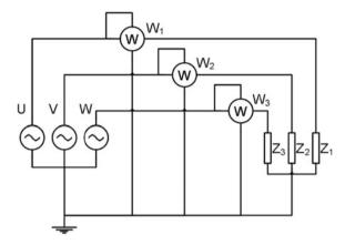
the voltage coil in parallel with the load. The three-phase circuits have some particularities due to load configurations.
