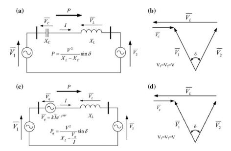
Fig. 8.26 Symmetrical system under series compensating,  $\mathbf{a}$  circuit diagram of series compensating capacitor,  $\mathbf{b}$  phasor diagram of capacitor,  $\mathbf{c}$  circuit diagram of SSSC,  $\mathbf{d}$  phasor diagram of SSSC
