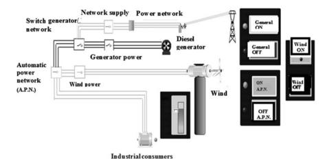
Fig. 15.3 SCADA system for hybrid EPS based on RESs
