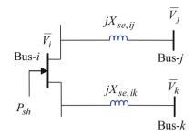
**Fig. 9.10** Equivalent power injection model of GUPFC
