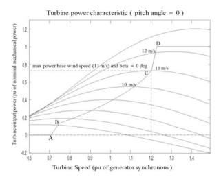
The reactive power control can be used to achieve the coefficient of ideal power in the DFIG connection point. When WTG feeds a strong power system, the reference reactive power can be adjusted for simplicity in zero. For the control of active power, the curve of feature of power-speed is used which is known as the curve of feature of absorption. [Calculations for the wind turbine power].
