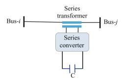
**Fig. 3.6** Unified Power Flow Controller (UPFC)
