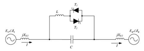
Fig. 8.16 Thyristor controlled series compensator
