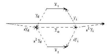
Fig. 1.10 Decomposition of an unsymmetrical system in three symmetrical systems
