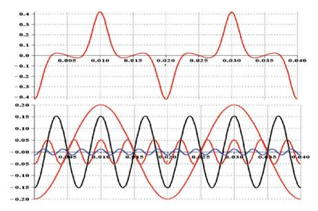
Fig. 1.28 Fourier series decomposition of a periodic distorted voltage signal
