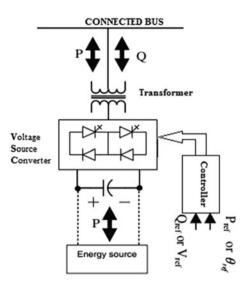
winding or thyristors control scheme. This control is very useful for the receivers, whose operations produce power surges in the electrical network.
