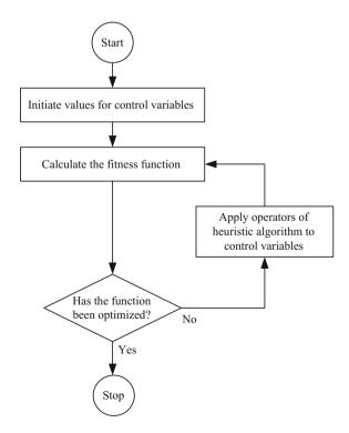
**Fig. 10.7** General reactive power optimization trend using intelligent algorithms
