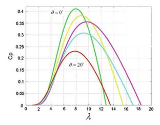
where  $C(\theta, \lambda)$  is the power coefficient of  $\theta$  angle of blades pace and  $\lambda$  is the ratio of speed of blade top to the wind speed. Figure 5.8 shows the method of change of power coefficient in terms of  $\lambda$  variable.
