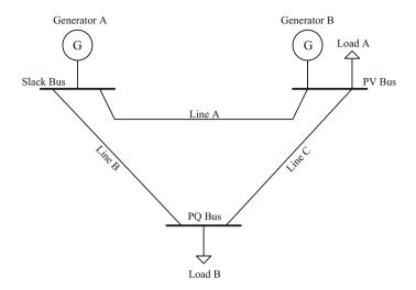
Fig. 10.1 Three-bus power system
