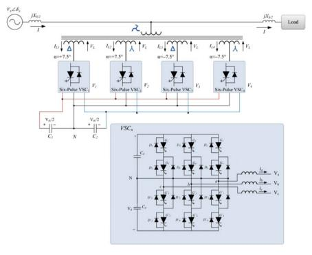
Fig. 8.22 Circuit diagram of a three-level 24-pulse STATCOM
