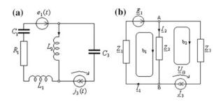
The computation of AC circuits is done using the complex representation. In complex domain, the passive elements are characterized by impedances and the energy sources by phasors. For the passive circuit elements, the impedances are computed as follows
