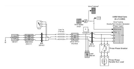
Fig. 5.4 Wind power plant system in MATLAB software
