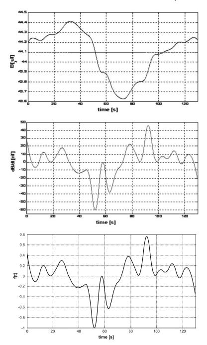
**Fig. 16.9** Course of the normal component of the magnetic induction  $B_n(t)$  depending on time (top), derivative of  $B_n(t)$  (middle) and f(t) (bottom)
