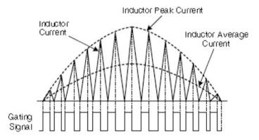
Fig. 4.38 Discontinuous mode of PFC operation
