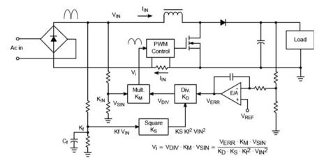
Fig. 4.37 Block diagram of the classic PFC circuit [68]
