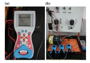
Fig. 1.25 a Power Q-meter, b Measurement stand
