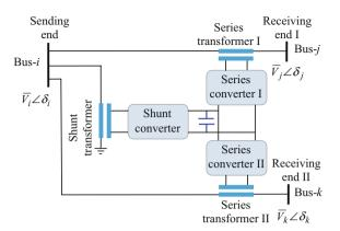
**Fig. 9.6** Voltage source model of GUPFC
