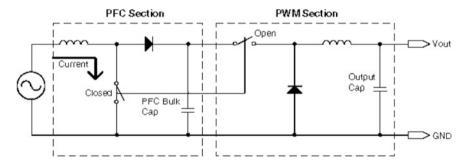
Fig. 4.43 Energizing the PFC Inductor [85]
