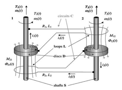
Fig. 16.4 Physical structure of the Rikitake dynamo
