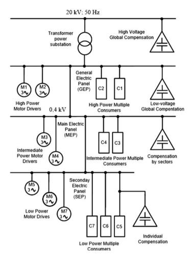
Fig. 2.18 Examples for placing the capacitors bank
