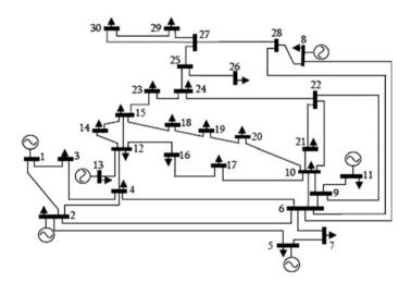
Fig. 5.9 IEEE standard 30-bus test system
