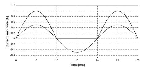
Fig. 4.31 Half-Wave rectified waveform test. Solid line—test waveform, dash line—reference waveform
