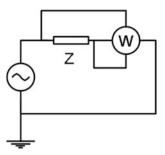
**Fig. 1.19** Active power measurement in three-phase circuits with neutral line load
