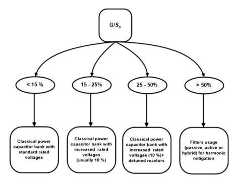
Fig. 2.23 Selecting the reactive power compensation possibility function of installation's nonlinear receivers' weight
