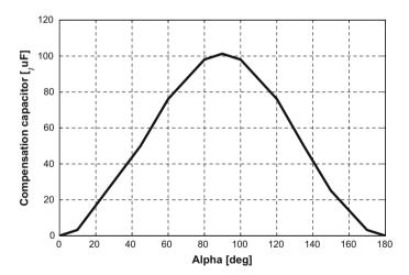
Fig. 4.12 Value of compensation capacitor versus alpha (Example 4.3)
