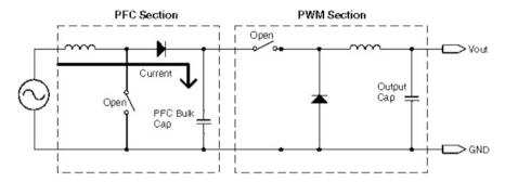
Fig. 4.41 Charging the PFC Bulk Capacitor [85]
