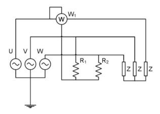
resistors as indicated in Fig. 1.23. The values of the additional resistors  $R_1$  and  $R_2$  are equal to the value of the resistance of the voltage circuit of the wattmeter.
