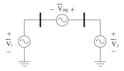
where  $\overrightarrow{V}_i$ ,  $\overrightarrow{V}_{inj}$  and  $\overrightarrow{V}_j$  are bus-*i* voltage vector, injected voltage vector by the series converter and bus-*j* voltage vector, respectively. By injecting an appropriate voltage vector by the converter, the voltage can be regulated.
