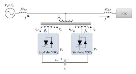
Fig. 8.20 Circuit diagram of two-level 12-pulse STATCOM
