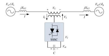
Fig. 8.25 Static synchronous series compensator (SSSC)
