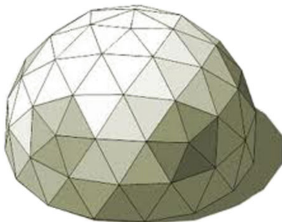
Fig. 1.40 Example of a geodesic dome (reproduced by courtesy of Lotus Domes UK)
